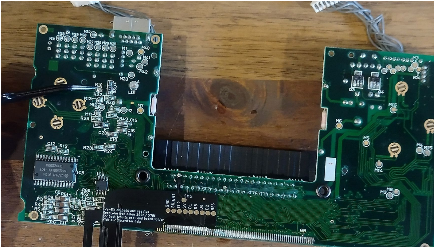
Locate pads M10 and M11. These are the Up and Down button signals.
