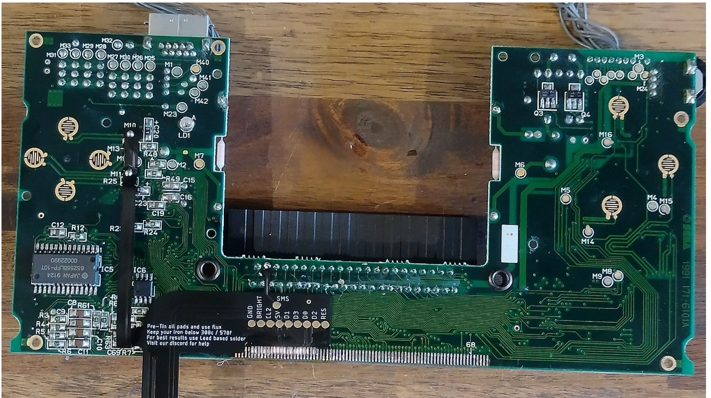
Fold the small ribbon back and solder down to M10 and M11.
