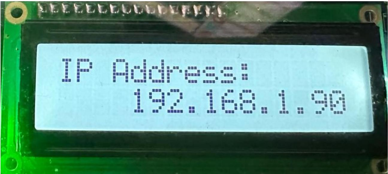
Once you have determined the switches IP address, open up a web browser on any device connected to your home network, and access the page at the switches IP address. In the example above, you would enter the web address [http://192,168.1.90](http://192.168.1.90)
