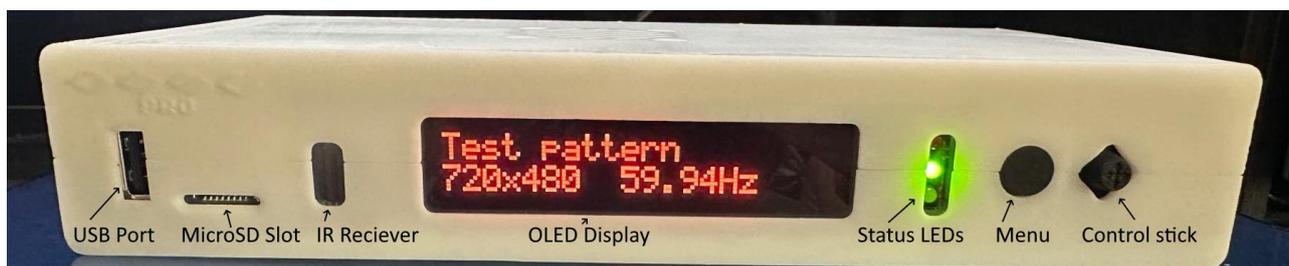
**USB Port** – For connecting and controlling external devices such as video switching hardware, or connecting accessories (note, these features are not currently available but may be added in future firmware updates).
