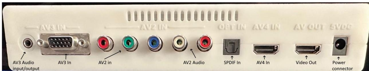
**AV3 Audio input/output connector** – This connector can be set to be an audio input (assignable to AV1, AV2 or AV3) or as an audio output/break out from AV1 SCART.
