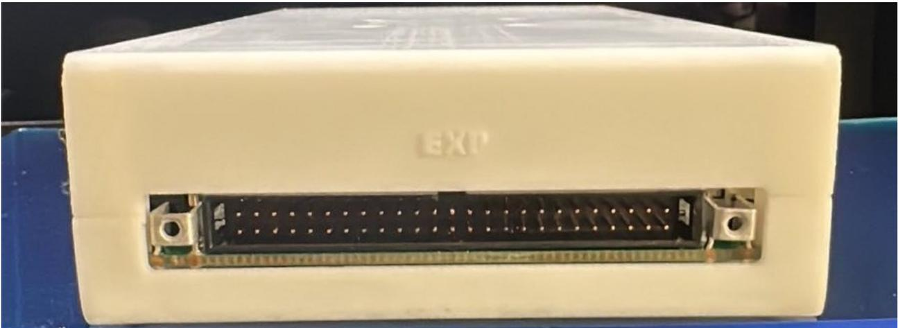
**Expansion Connector** – For adding expansion boards to the OSSC Pro. Expansion boards can add new functionality and input and output options.
